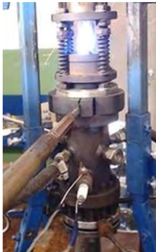
Tested system - Dnipro / Promin Aerospace perchlorate ammonium / polyethylene
